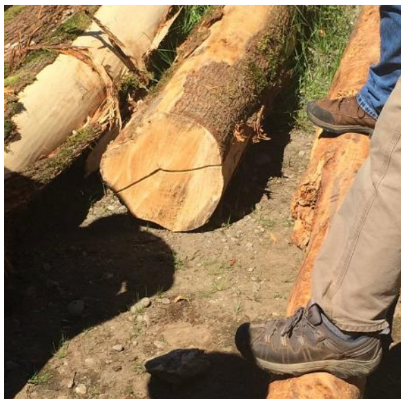
Figure 6. This log has a split. Since it is mostly vertical it may not endure a deduction because when the log is processed the mill may be able to cut the log along the split. If the split is long and jagged or on a curve, then a length deduction can occur.
