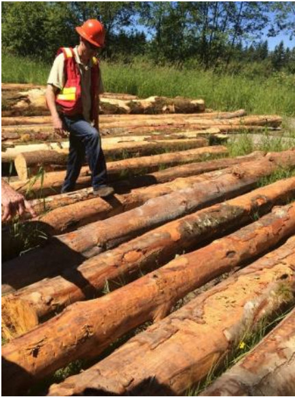
Figure 1: This is a log scaling yard. The logs are lined up after they are felled and processed. The scaler will walk down the line assessing damage and take deductions where necessary. In the bottom right of this photo there are two logs that have a series of nicks along the length of them. This is a result of the mechanical damage from the processor's feeding wheels. Try and encourage your loggers to stay away from steel feeding wheels in their processors if possible. Rubber wheels are the best for hardwoods. These nicks cause compaction in the wood and are visual defects in the finished alder boards. This decreases the quality of the processed wood to a paint grade board and could mean a quality deduction depending on the type of sale you are doing. Additionally, if these nicks become deep enough then they can result in a diameter deduction as well.
