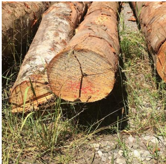
Figure 5. This is an example of cross break, where the log is split vertically and horizontally. This could result in a length deduction for the length of the split depending on the severity of the break.
