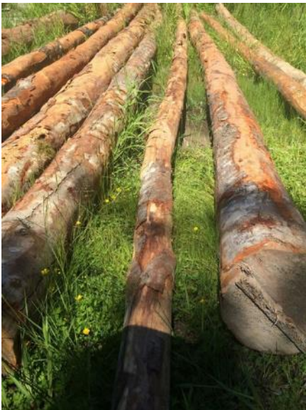
Figure 2. Sweep or crooks can cause length deductions in the logs. There is no deduction as long as the log scaler can run a tape measure along the length of the log without it leaving the log's surface. If it does leave the log's surface then the scaler will consider it 2 or more logs - depending on the number of sweeps and crooks - and then deduct the length of the
